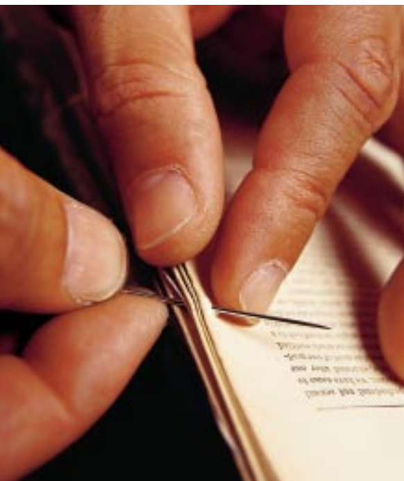
Not for rough hands: The pages are stitched together with needle and thread.
